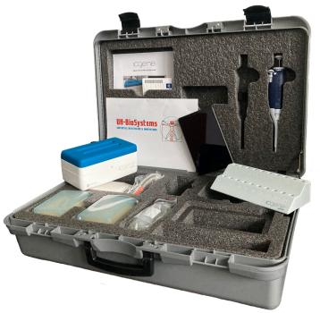
Up to 48 samples can be analyzed using the real-time fluorescence amplifier, which is operated via a user-friendly Android interface.
